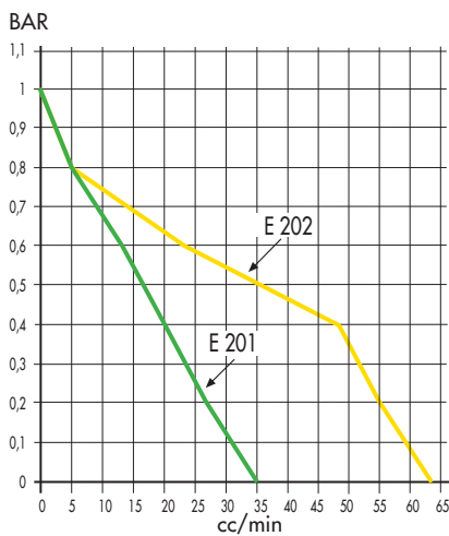
E 201 - E 202 "Dosatrici" "Dosing pump"
